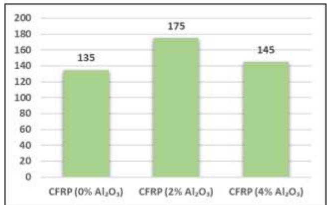
Fig 4: Flexural strength variation as the weight percentage of Al 2 O 3 increases
