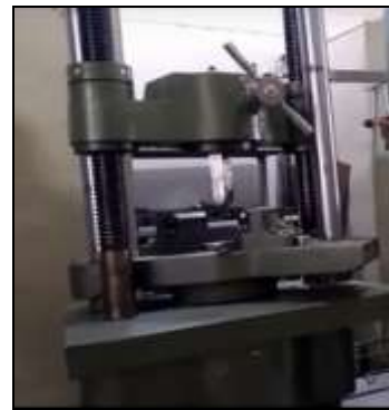
Fig 3: Setting up for flexural testing
