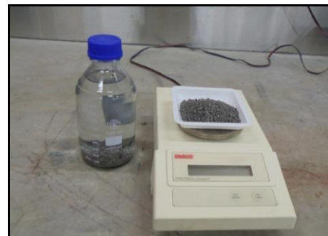
Fig 3: Weighting of 100-grams (right) prior to the sample being added to the bottle extractor (left) containing 1 - litre of distilled water
