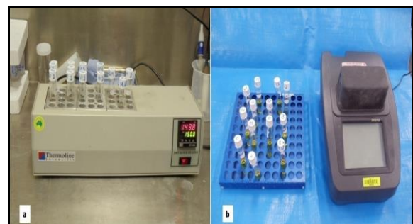
Fig 7: (a) vial heater, (b) COD photometer
