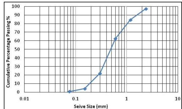
Fig 1: Particle size distributions (sieving method) of Colga double washed sand
