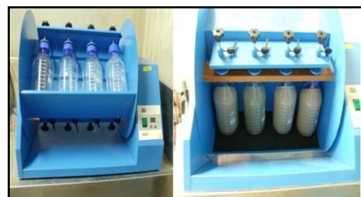
Fig 4: Rotary agitation device used for sample extraction
